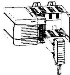
2. Press quickly and evenly to seat the RTB on the module until the latches snap into place.
