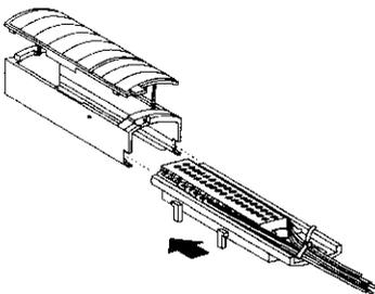
**IMPORTANT** If additional wire routing space is required for your application, use the extended-depth housing, catalog number 1756-TBE.
